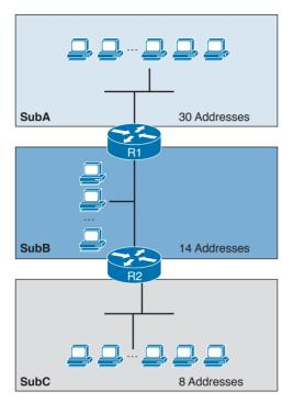
Figure 1-50 Example of Three Subnets with Different Requirements for IP Addresses
