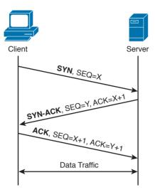
Figure 1-82 TCP Three-way Handshake
