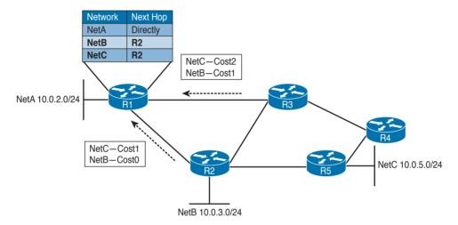
**Figure 1-59** *Example of a Distance Vector Exchange*
