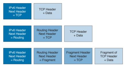
Figure 1-68 Chained Extension Header
