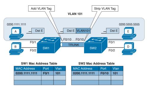
**Figure 1-29** Example of a VLAN and VLAN Trunk Used on a Topology with Multiple Switches
