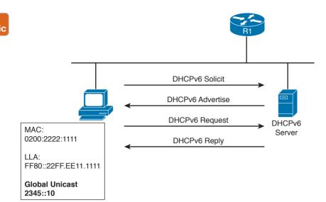
Figure 1-77 Stateful DHCPv6 Exchange for IPv6 Address Assignment
