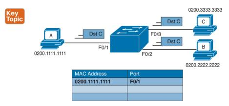
**Figure 1-20** Example of a MAC Address Table Being Updated as the Frame Is Received and Forwarded by the Switch
