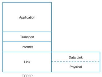
Figure 1-1 TCP/IP Stack Model
