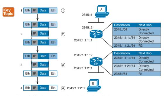
Figure 1-66 Communication Between Hosts Using IPv6
