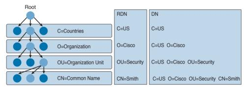
Figure 5-4 Comparing Distinguish Name (DN) and Relative Distinguish Name (RDN)
