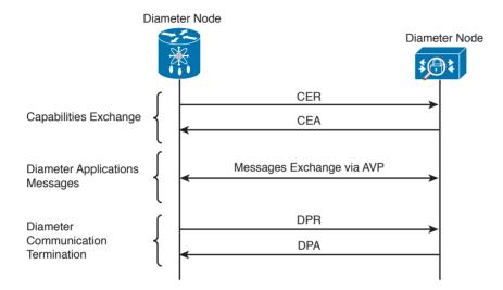
Figure 4-15 Diameter Capability Exchange/Communication Termination
