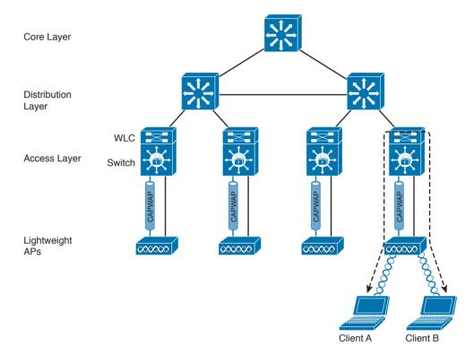
Figure 1-41 Converged WLC Architecture
