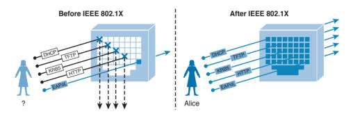
Figure 14-17 Traffic Allowed Before/After 802.1x Authentication and Authorization
