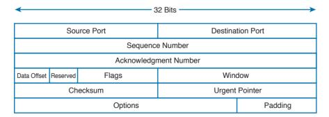
Figure 1-81 TCP Header Structure
