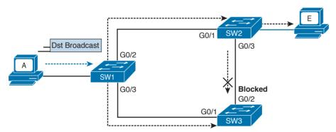
**Figure 1-25** Example of Layer 2 with STP Enabled
