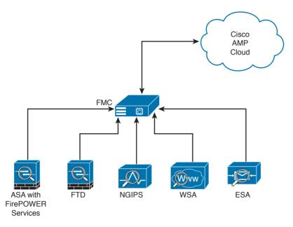
Figure 2-14 AMP Connectors Communicating to the FMC and the Cloud
