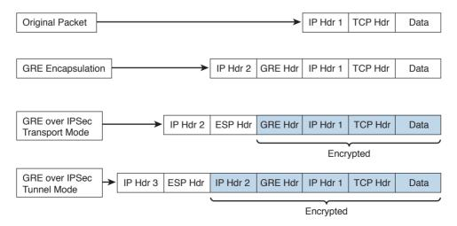
Figure 7-5 Transport Mode vs. Tunnel Mode in IPsec
