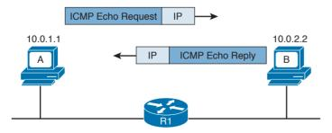
**Figure 1-62** *ICMP Echo Request and Echo Reply Exchange*
