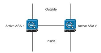
**Figure 2-7** *Firewalls in Active-Active Failover Mode*
