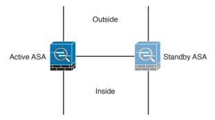
Figure 2-6 Firewalls in Active-Standby Failover Mode
