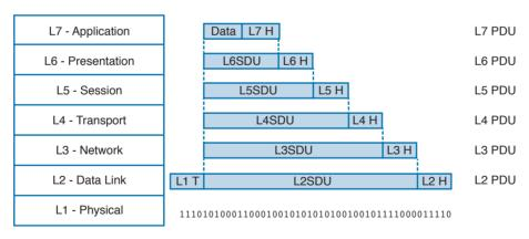
Figure 1-7 Encapsulation in the OSI Model
