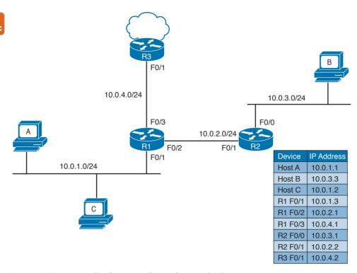
Figure 1-56 Example of a Network Topology with Three Routers
