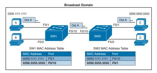
**Figure 1-23** Frame Forwarding and MAC Address Table Updates with Multiple Switches. Host E replies to a frame sent by Host A.
