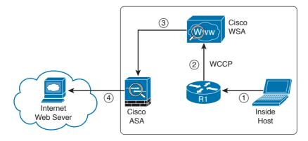
Figure 2-16 WSA Transparent Proxy Configuration
