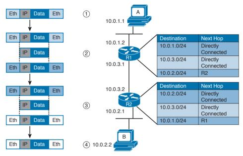
Figure 1-43 Example of IP Packet Routing and a Routing Table
