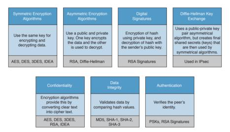
**Figure 6-6** Fundamental Encryption Components
