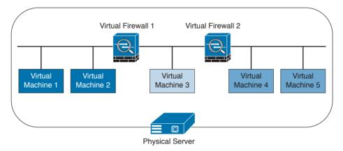
Figure 2-11 Virtual Firewalls Example
