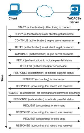
Figure 4-14 TACACS+ Message Exchange for Authentication, Authorization, and Accounting
