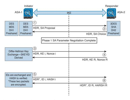
**Figure 7-3** *IPsec Phase 1 Main Mode Negotiation*
