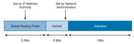
Figure 1-70 Global Unicast IPv6 Address
