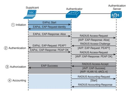
Figure 4-19 802.1x Port Access Control Exchange
