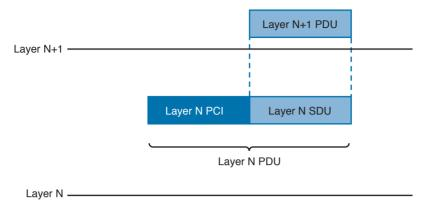
Figure 1-6 Relationship Between PCI, PDU, and SDU
