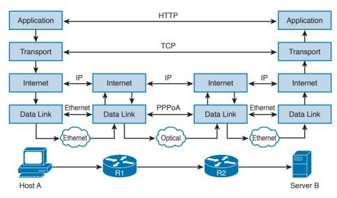
**Figure 1-4** *Interaction of the TCP/IP Model Layers*
