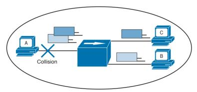
Figure 1-14 Collision Domain with a Hub or Repeater
