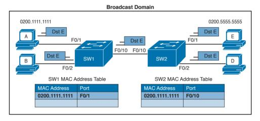
**Figure 1-22** Frame Forwarding and MAC Address Table Updates with Multiple Switches. Host A sends a frame for Host E.
