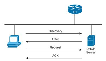
Figure 1-53 Basic DHCP IP Address Assignment Process
