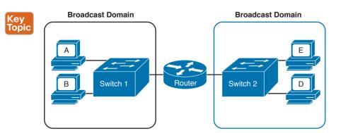
Figure 1-19 A Router Dividing the Network into Two Broadcast Domains
