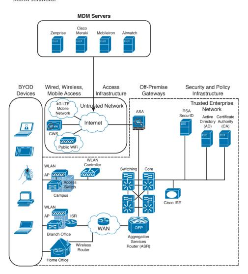
**Figure 5-15** Cisco ISE Integration with Cloud-Based MDM Solutions
