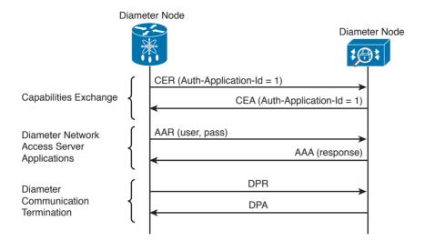
**Figure 4-16** Diameter Exchange for Network Access Services
