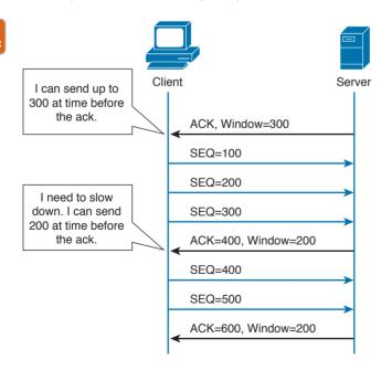
**Figure 1-86** Example of TCP Flow Control
