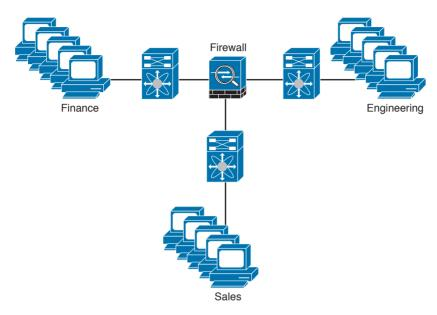
**Figure 2-5** Firewall Providing Network Segmentation
