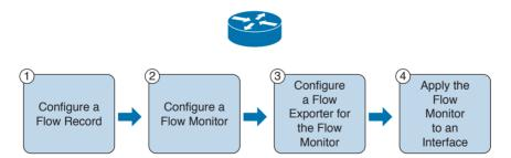
Figure 11-24 Flexible NetFlow Configuration Steps
