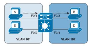
Figure 1-33 Inter-VLAN Flow with a Multilayer Switch
