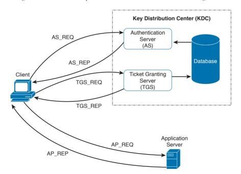
**Figure 5-7** Authentication and Authorization Using Kerberos
