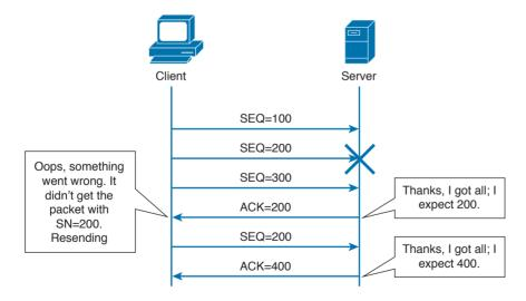
**Figure 1-85** *TCP Error Detection and Recovery*
