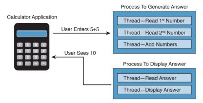
**Figure 8-1** *Calculator Process and Thread Example*
