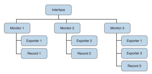
Figure 11-23 Flexible NetFlow Model
