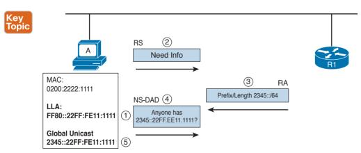
Figure 1-76 Address Assignment via SLAAC
