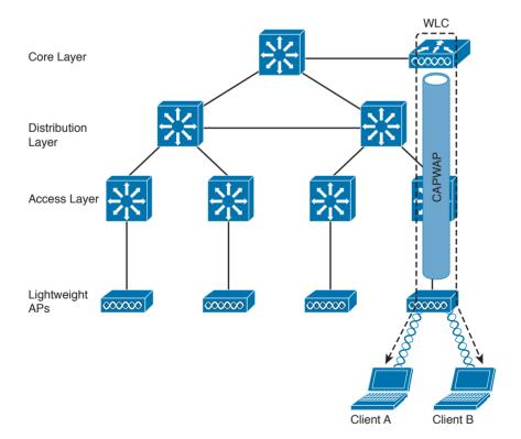
Figure 1-40 Centralized WLC Architecture
