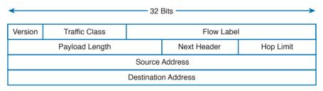
Figure 1-67 IPv6 Header
