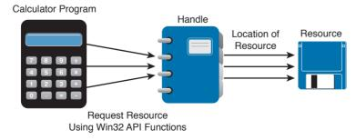
**Figure 8-6** Calculator Example Showing Handles
