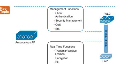
Figure 1-39 Comparison Between an Autonomous Access Point and a Lightweight Access Point
