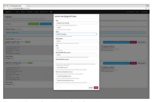
Figure 11-10 Launching a New Graylog Syslog UDP Input
