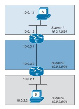
**Figure 1-47** Example of Addressing in a Topology with Three Subnets
