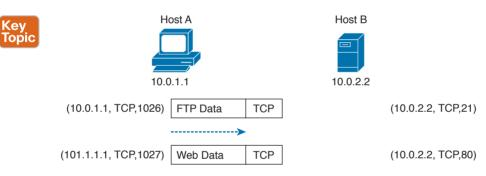
Figure 1-79 Example of TCP Multiplexing
