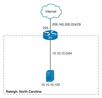
Figure 11-25 Flexible NetFlow Model
