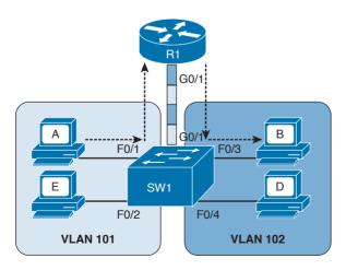
Figure 1-32 Router on a Stick (ROAS)
