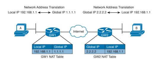
**Figure 1-52** Using NAT to Allow Communication Between Two Hosts with the Same IP Addresses Belonging to Two Different Organizations
